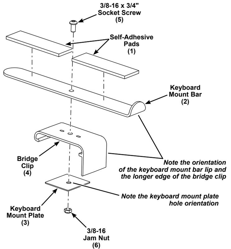
3. Attach the assembled keyboard mounts to the bridge extrusion by inserting the short sides of the bridge clips into the outside groove. Press down to snap the long sides of the bridge clips into place.
